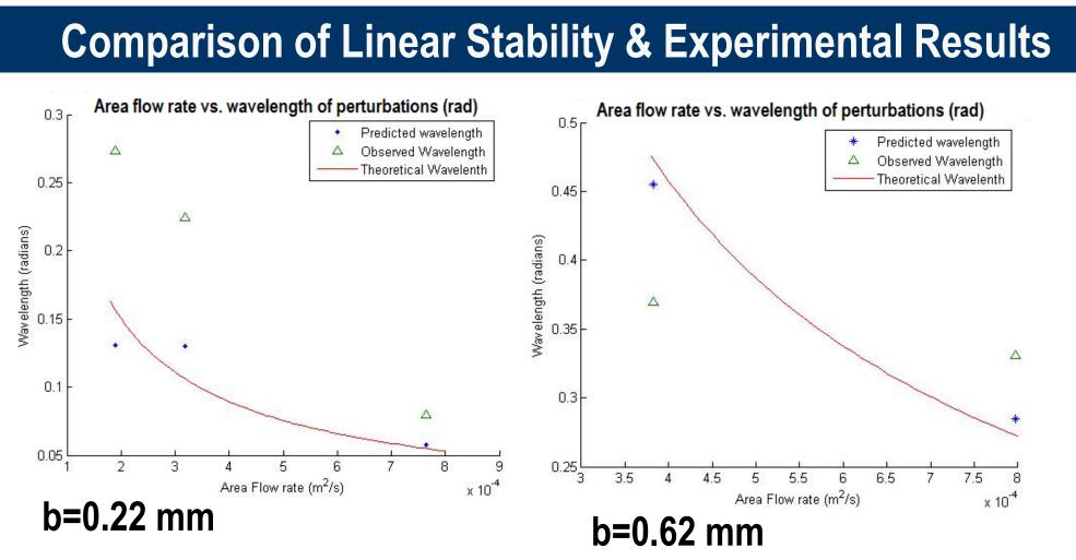
Above we see comparison of linear stability and experimental results as a function of flow rate for two different separation distances between the plates, b.
