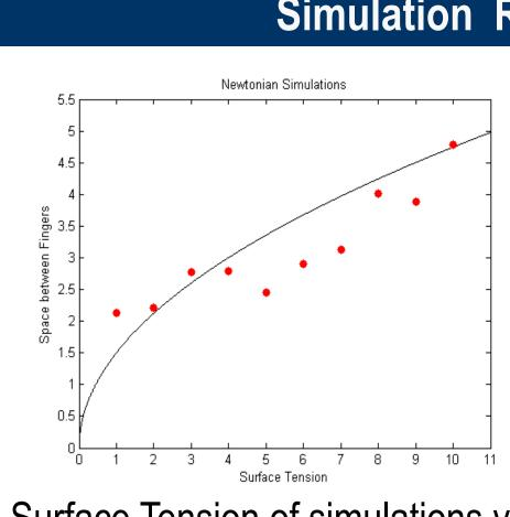
Surface Tension of simulations vs. space between fingers compared to a square root relation as seen in linear stability analysis.
