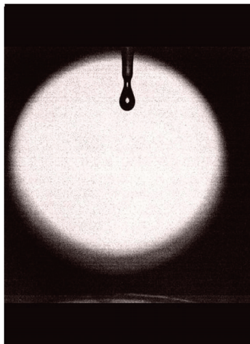
Figure 3: Snapshot of a break-up process using high speed camera (20,000 frames per second).
