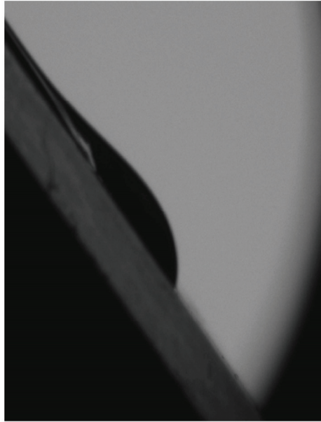
Figure 2: Profile of a milimetric fluid strip sliding down an incline.
